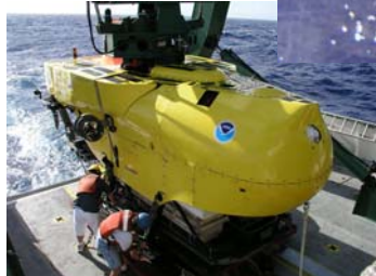
The Pisces V submersible can hold up to three people. It weighs 13 tons and has a maximum operating depth of 6,280 ft.
