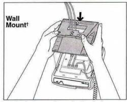
Lower the stand into the slots on the base of the telephone, as shown in the desk or wall mount illustration above.
