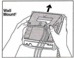
Slide the stand back until it clicks into the locked position, as shown in the desk or wall mount illustration above. The excess line cord fits into the stand of the telephone.
