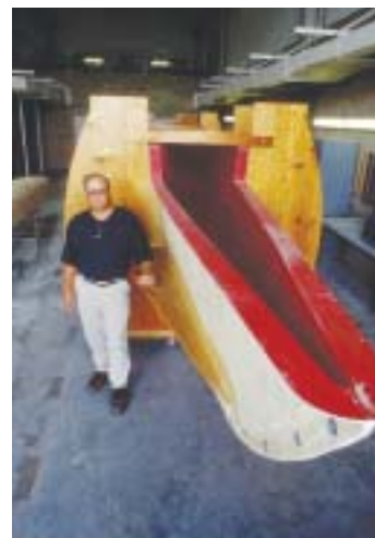
Honolulu CC Instructor Robert Perkins with mold for canoe hull
