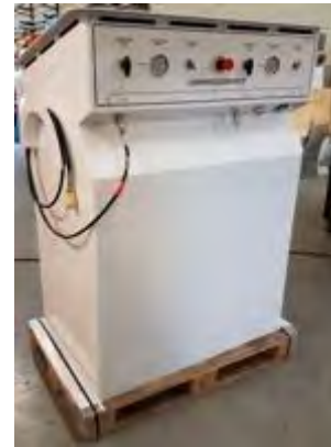
Figure 7. MTA Boost Compressor Fueling Post.
