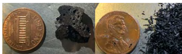
Figure 2. Transient plastic phase biocarbon (left) and non-transient plastic phase biocarbon on (right). Both products made from the same biomass feedstock.
