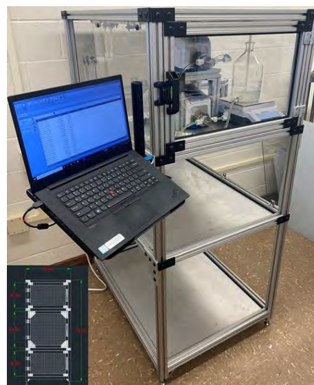
Figure 1. HNEI fabrication and optimization of a forward osmosis water flux testing system.
