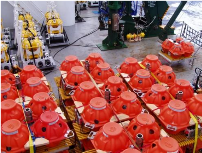
SIO (yellow) and WHOI OBS (orange) data acquisition systems stored for transit on the launch deck of the R/V Kilo Moana. Photo credit: Gabi Laske, SIO/UCSD
