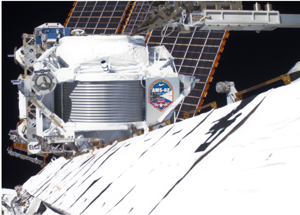
Figure 1. From its vantage point \sim 240 miles (400 km) above the Earth, the Alpha Magnetic Spectrometer (AMS) collects data from passing cosmic rays from primordial sources in the universe before they pass through the Earth's atmosphere.
