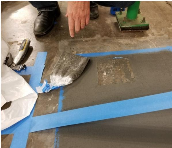
*Contractor's Conduction Pull Test on Traffic Coating Mockup*
