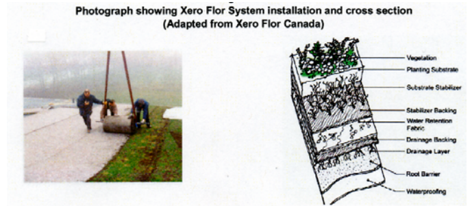
Photograph showing Xero Flor System installation and cross section (Adapted from Xero Flor Canada) Photo courtesy of http://www.hrt.msu.edu/greenroof/
