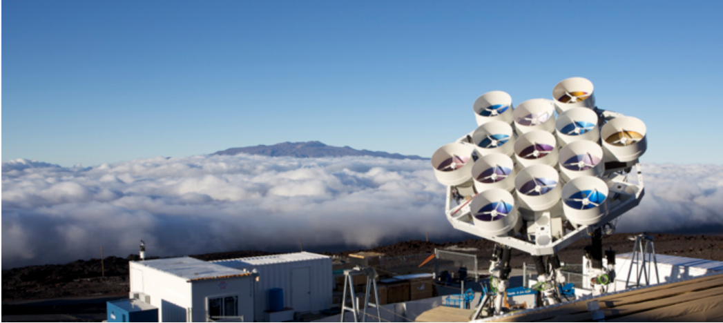
Figure 2: AMiBA with thirteen 1.2m antennas was completed in the end of 2009. The 13-element array, with improved resolution and sensitivity, can effectively study galaxy clusters that are much further away from us. The summit of Mauna Kea is shown in the background.
