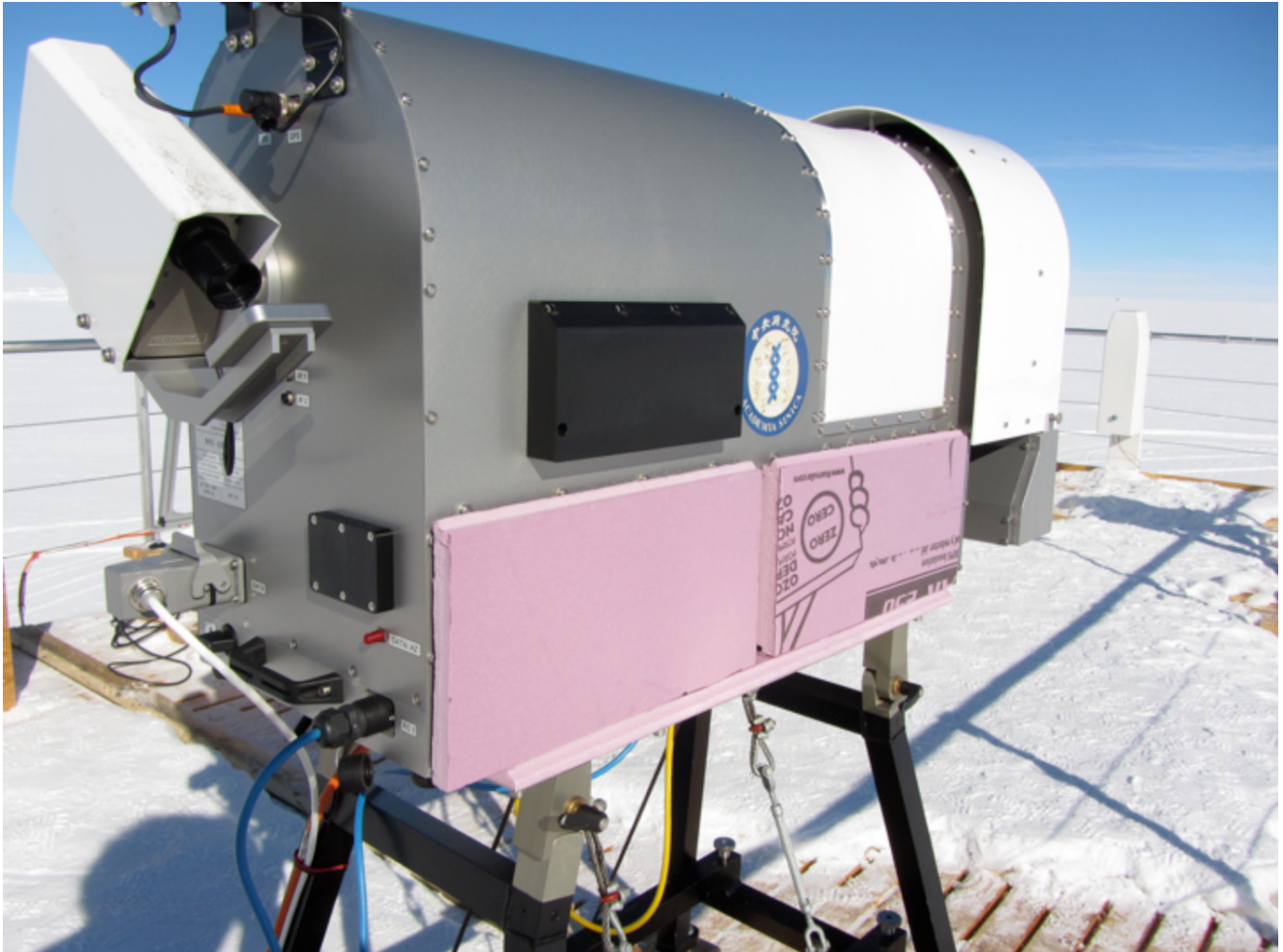
Figure 3: A site surveying radiometer for the GLT project was deployed to the summit of Greenland in 2011. This instrument is to measure the atmosphere clarity of the site.
