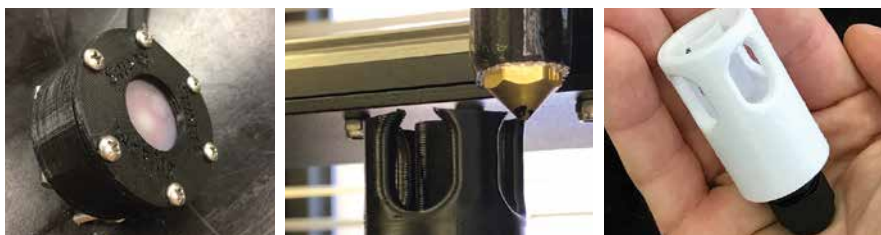
LEFT: A low-cost custom submersible pressure sensor for measuring tides and waves. MIDDLE: 3D printing technologies allow for rapid, low-cost prototyping of sensor designs. RIGHT: A completed sensor cage: costs $0.18 in materials, takes only 40 minutes to build, and stands ready for embedding of a high-resolution temperature sensor for coral bleaching studies. PHOTOS: BRIAN GLAZER
