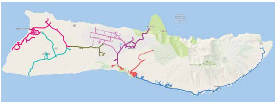
A schematic representing the detailed grid models of Molokai’s distribution circuits developed by the GridSTART team to assess the impacts of high penetrations of renewable energy.
